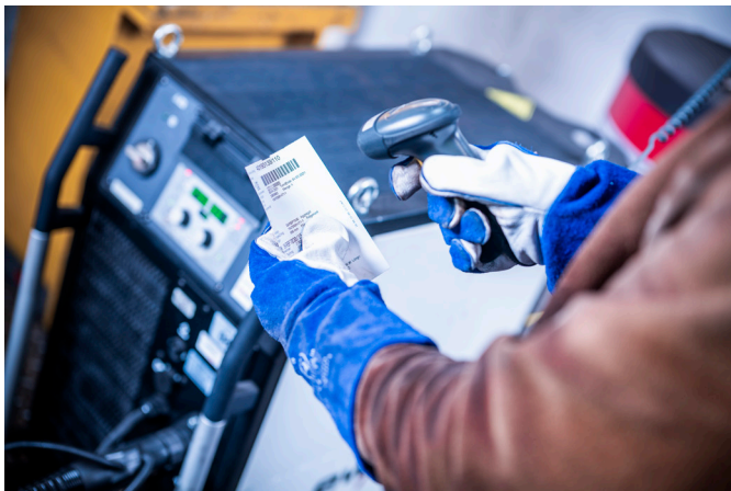
The Xbutton contains all information about welding procedures and parameters. This also allows the verification of the welder's identity.
